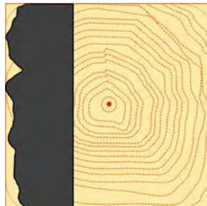
Charring on the exposed face of a 6x6 after 1-hour
